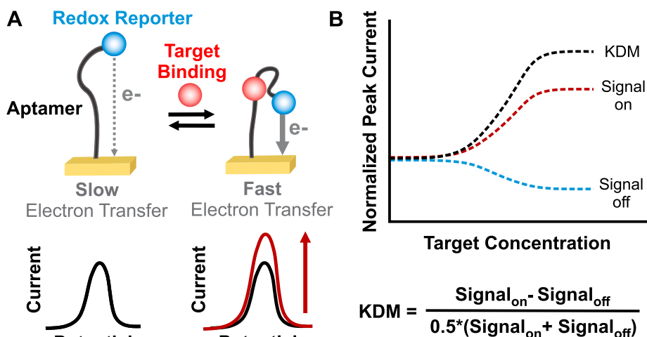
Fig. 1. (A) Most commonly, electrochemical aptamer-based (EAB) sensors consist of an aptamer (black) modified with a redox-reporter (blue) attached to a gold electrode (yellow). Upon binding of target (red), a change in electron transfer kinetics between the redox reporter and the surface occurs, which is easily monitored using square wave voltammetry as an increase (or decrease) in square wave voltammogram peak current (red). (B) Depending upon the square-wave frequency employed, the peak currents seen in square wave voltammetry can increase ("signal on" behavior) or decrease ("signal off") in response to target binding. To assess target binding, we titrate the sensors with known amounts of target, and measure the response at different square wave voltammetry frequencies. To increase gain and correct for the appearance of drift, we obtain Kinetic Differential Measurement (KDM) values by taking the difference in normalized peak currents collected at a signal-on and a signal-off frequency, then dividing that value by the average of the normalized signal-on and signal-off peak currents (detailed in section 2.5) (Ferguson et al., 2013).
